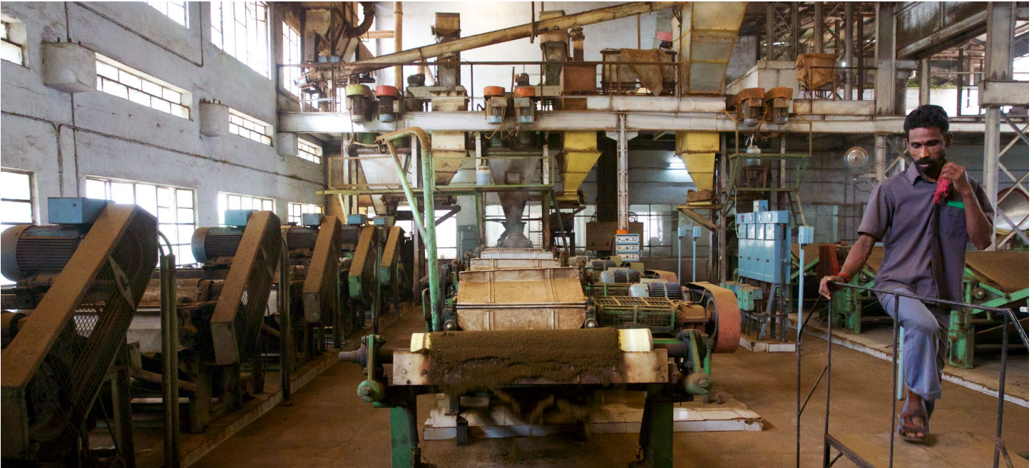
The Semni Valley Tea Estate factory has 4 CTC lines, two of which are shown here.
